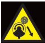
Caution! The tool can contact to a voluminous material. Loss of control and injuries can be created.
